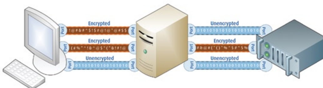
EpiForce policy-based encryption will enable data communications between servers and clients and between servers to be selectively encrypted by port to increase security administrator flexibility.
